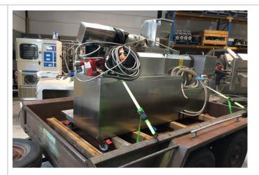
Figure 22 The extruder was seated on the timer frame to avoid moving around during transportation.
