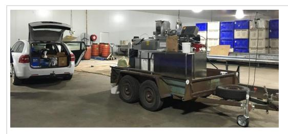
Figure 25 Extruder is set up on arrival at the site and connected to power and water supply.
