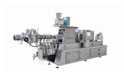
Figure 11. Photograph of CSIRO Pilot Scale Extruder
