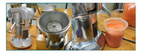
Figure 3 First juice extraction for preparation of pomace1
