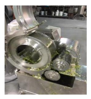
Figure 5 Machine used for dicing the broccoli and carrots
